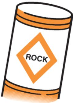
**DIAMOND SHAPE** warns of Danger. Wording appearing in diamond includes ROCK, DAM, SNAG, DREDGE, WING-DAM, FERRY CABLE, MARINE CONSTRUCTION, WRECK, etc.
