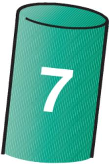
**ALL-GREEN BUOY** indicates vessels should pass between it and its companion, an all-red buoy. Keep green buoy on port (left) side when proceeding upstream, or when entering a channel from the main body of water.
