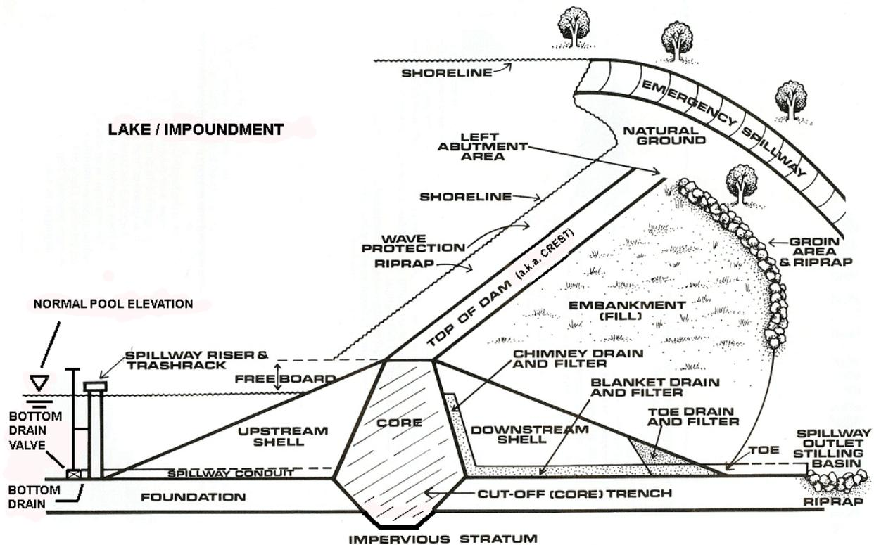
**Figure 2 – Parts of an Earthen Dam (from Dam, Operation, Maintenance, and Inspection Manual – NCDENR Land Quality Section)**
