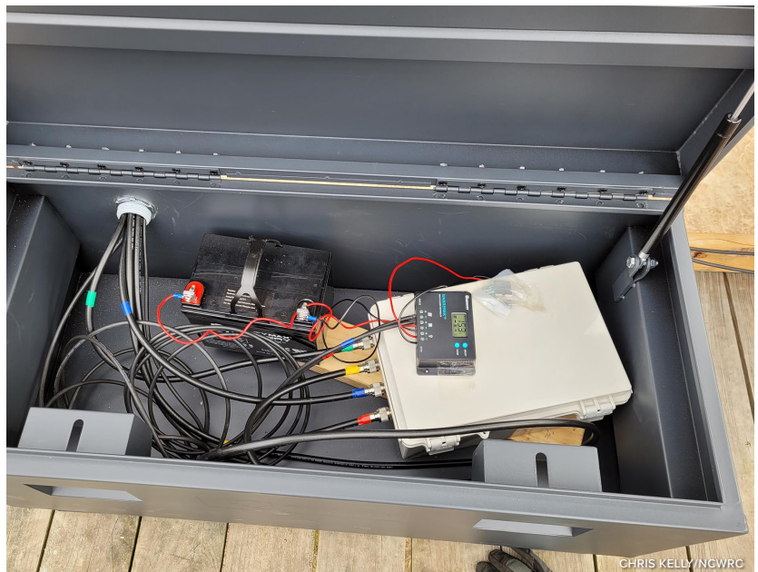
The Sensor Station, 12 V battery, and charge controller are housed inside a locked steel box, which is bolted to the platform.
