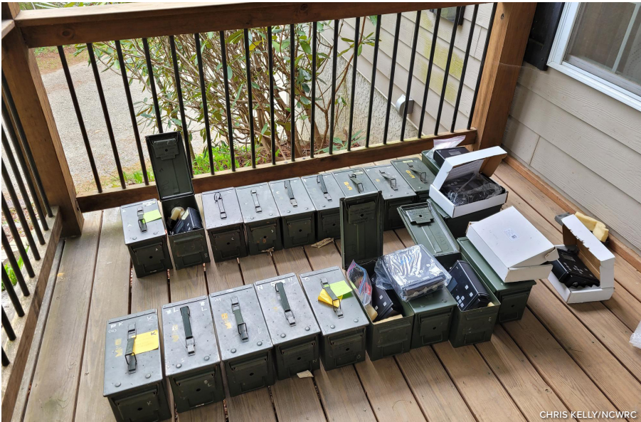
Above left: NCWRC staff prepared a fleet of Pettersson D500 ultrasonic detectors for Virginia Tech researchers to deploy for the Carolina northern flying squirrel occupancy monitoring program. Autonomous recording units have been shrinking from the hefty Petterssons housed in 50 caliber ammo boxes to deter bear damage to tiny AudioMoths, above right (they're even wearable!). Miniaturization of equipment makes it feasible to haul more ARUs farther into the backcountry. Regardless, staff and partners make it happen (below).
